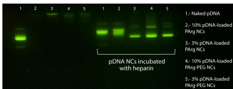
Figure 3: Gel electrophoresis of naked pDNA, pDNA-loaded PARG nanocapsules and pDNA-loaded PARG-PEG nanocapsules at 3% and 10% loading pDNA/nanocapsules, without and after treatment with heparin.
