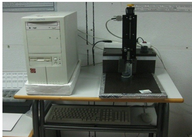
Figure 2.2: Dip-Coating instrument composed of a micrometer optical platform aligned in the vertical position and controlled by a PC with conventional software.
