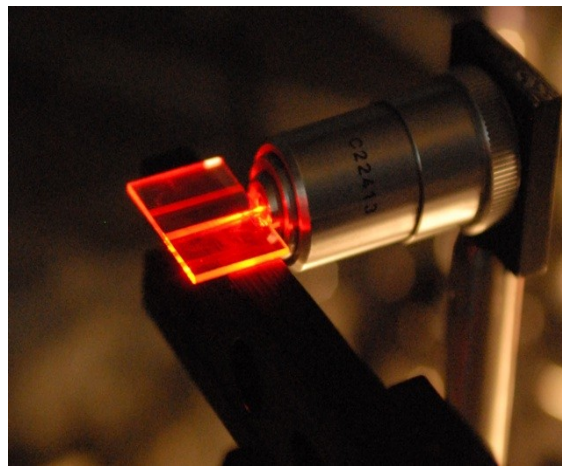
Figure 3.92: Demonstrative photograph showing how light from a He-Ne laser ( \lambda=632.8 nm, 1 mW) is guided through a 63Cu37Zn brass derived LAB diffusive waveguide.
