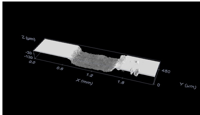
Figura 3.30: Image obtained by confocal microscopy of the surface of a channel engraved via laser ablation of one planar commercial glass substrate.
