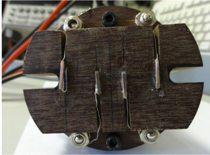
Figure 2.25: Specifically built four-point resistance probe for electrical resistance measurements [courtesy of L.A. Angurel at Instituto de Ciencia de Materiales de Aragón, ICMA-CSIC].
