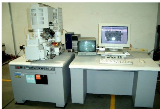
Figura 2.17: Image of a commercial Scanning Electron Microscope (SEM) where the electron acceleration column and observation chamber are on the left and the computer control is on the right side.
