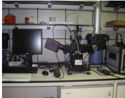
Figure 2.29: Image of the spectral Woollan M2000U ellipsometer used in this work for the characterisation of Sol-Gel films.
