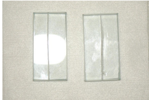
Figura 3.27: Image of mechanically engraved channels obtained on soda lime commercial glass substrates.
