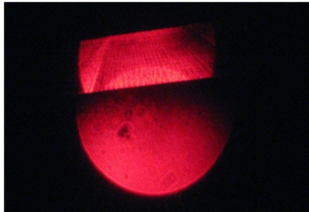
Figure 3.91: Projected image of a waveguide output showing some modulation of the light passing through a 63Cu37Zn brass derived LAB sample.
