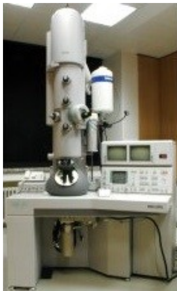
Figura 2.19: Photograph of a commercial Transmission Electron Microscope (Philips CM300FEG/UT-STEM) located in Bonn and used for this study.
