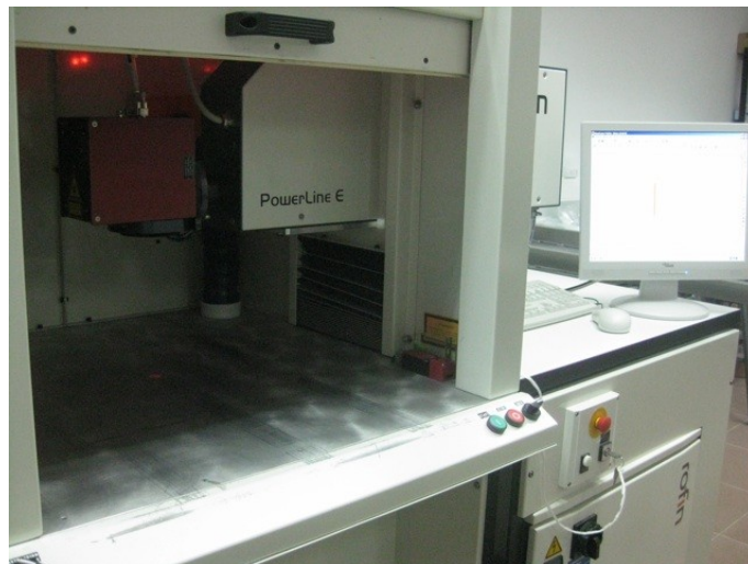
Figure 2.7: Powerline E model 20W Nd:YVO4 laser manufactured by Rofin®. The galvanometer head is enclosed within the red box on the left side of the photograph, placed at the resonator output and within a safety enclosure.
