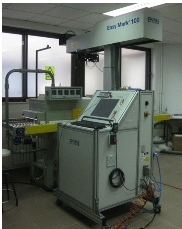
Figure 2.5: Image of the CO 2 laser system (EasyLaser) coupled to a roller kiln (Nannetti), used in the present work and patented by Estepa and de la Fuente [81].
