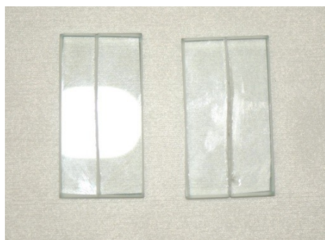
Figura 2.14: Image of mechanically engraved channels onto a commercial glass substrate.
