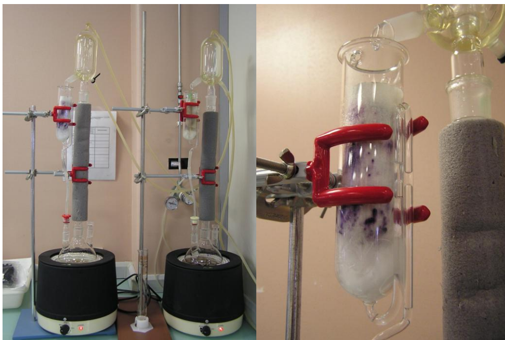
Fig. 6.1. The modified Soxhlet extractor for simulating geochemical weathering of biochar.
