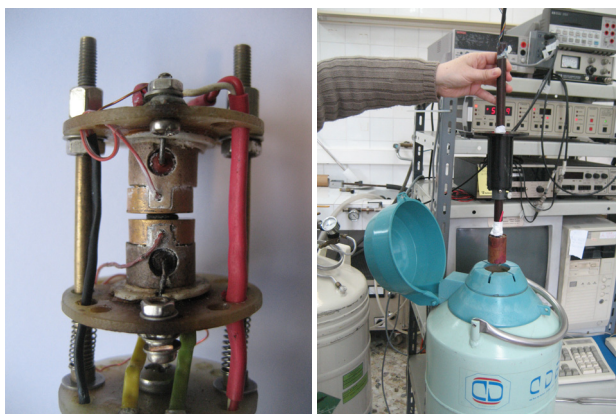
Figure 2.3: (Left) Detail of the home-made sample holder used in the thermoelectric power measurements. Cold pressed pellets are placed in between two gold-plated copper blocks. A thermal gradient of \pm 1 K is established between the copper blocks. (Right) The sample holder is protected and introduced in a dewar containing liquid nitrogen that provides a cold bath for temperature control.
