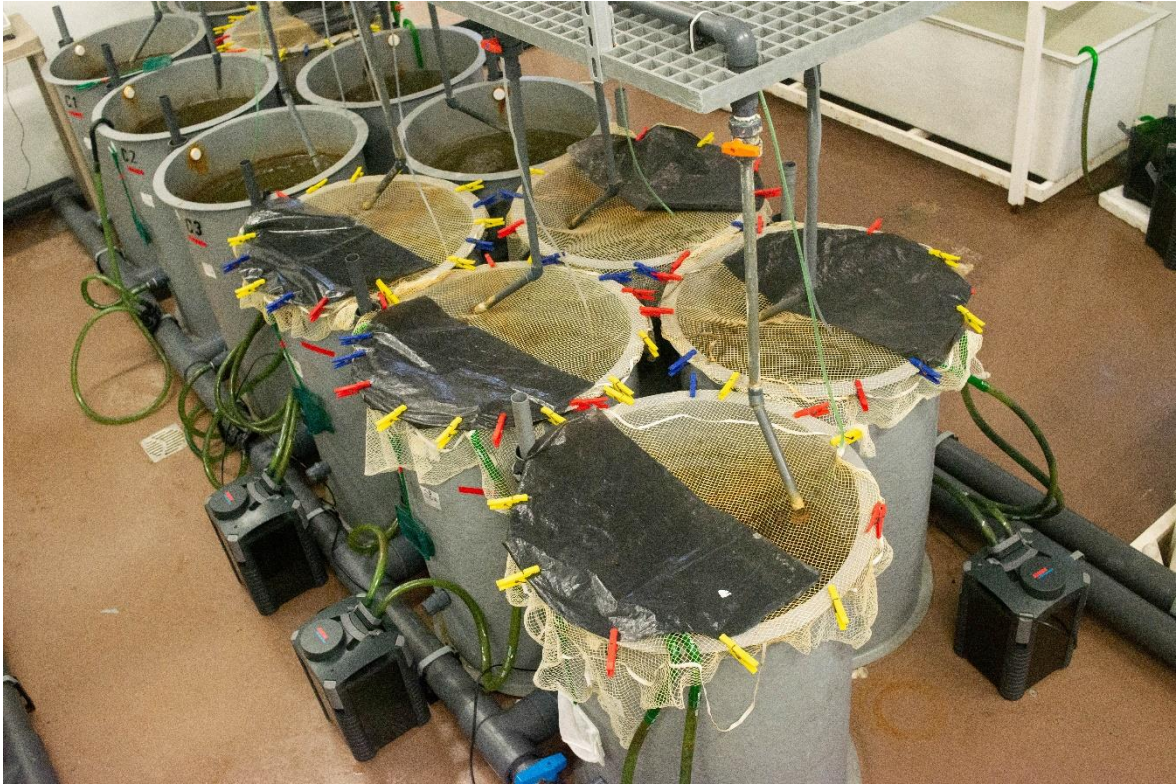
Figure 9. Closed water system tanks fitted with Eheim 350 Experience external canister filters. Photo by Tiago Lourenço.
