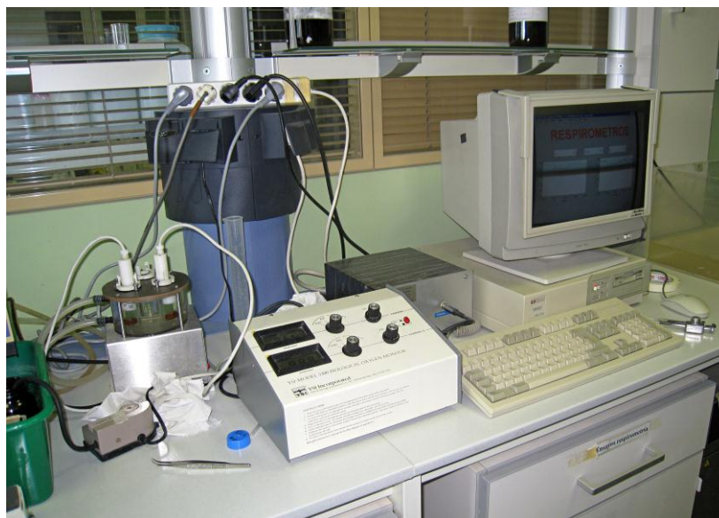
Figure 2.6 Respirometric system: left, thermostated test cells; center, biological oxygen monitor; right, data acquisition system.
