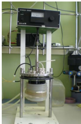
Figure 4.1 Autotrophic denitrifying SBR.
