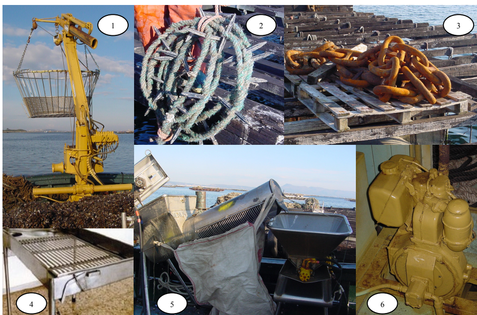
Figure 3.5. Some inventoried elements: (1) hydraulic crane and basket, (2) rope with plastic pegs, (3) shackle chain, (4) grading table, (5) de-clumping machine, re-tubing machine and big-bag, (6) engine
