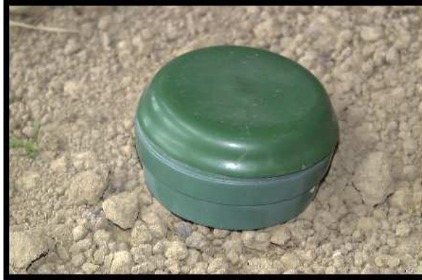
Figure 1.9: A typical low metal antipersonnel mine (Type 72).
