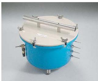
Figura V.1. “Olla extractora”<sup>32</sup>
