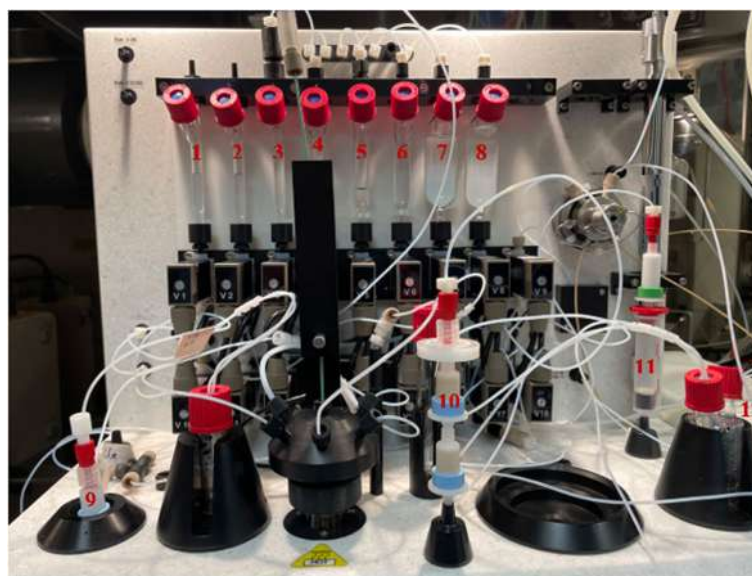
Fig. 5 GE TRACERlab™ FXFN module set-up of reagents and cartridge/filter assembly for the radiosynthesis of [^{18}\text{F}] FSPG
