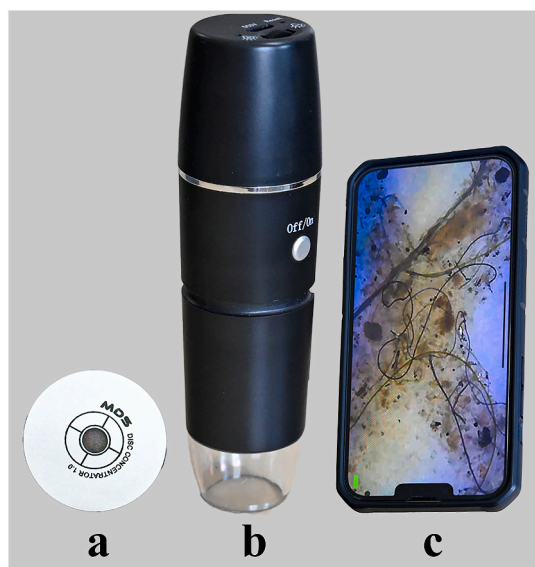
Fig. 3. Microfibres Detection System (a – sampling filter; b – microscope; c –smartphone).
