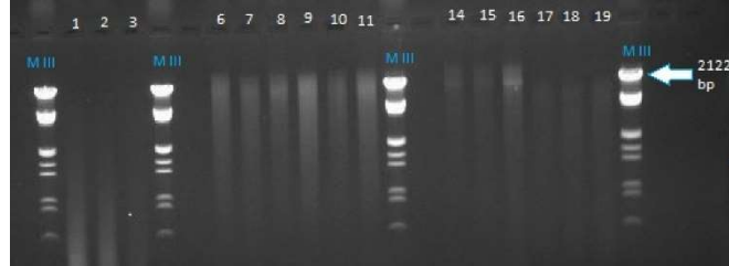
Figure A1.2. Picture of agarose gel. M III, DNA ladder with upper band (~21,226 bp) indicative of high molecular weight DNA. Sample 1-3: buckwheat pollen, Sample 6-11: sunflower pollen, Sample 14-19: dandelion pollen
