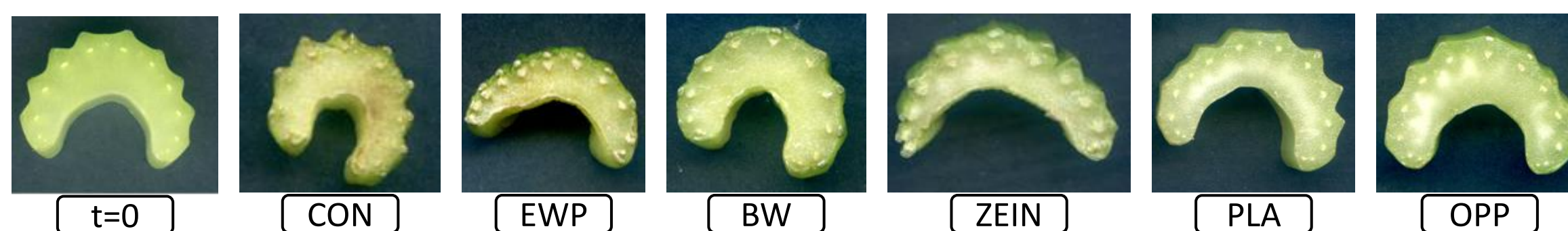
Figure 3. Scanned images of fresh-cut celery packaged in bags made of EWP and commercial films, after 14 days of storage at 5°C.
