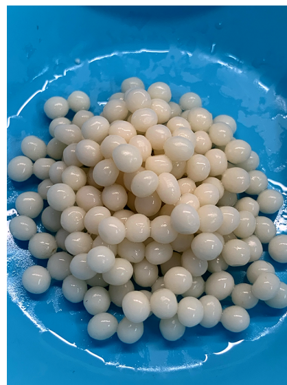
Figure 1. Cells of Komagataella phaffii entrapped in calcium alginate. Small spheres of about 3 mm diameter were obtained.
