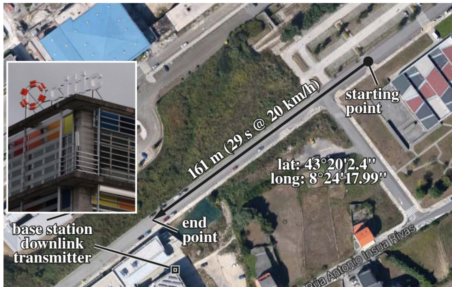
Figure 4.7: Measurement scenario considered for the Time-Division LTE (TD-LTE) measurements in A Coruña, at the University of A Coruña. The path followed by the receiver as well as the location of the transmitter are indicated in the figure.
