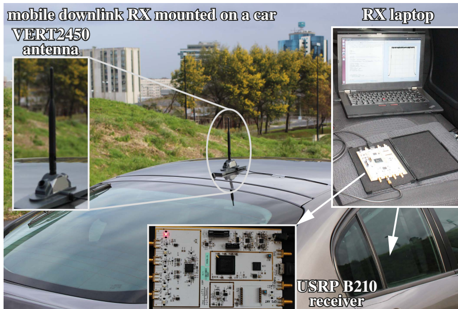
Figure 4.5: GTEC Testbed node acting as a mobile receiver mounted on a car.
