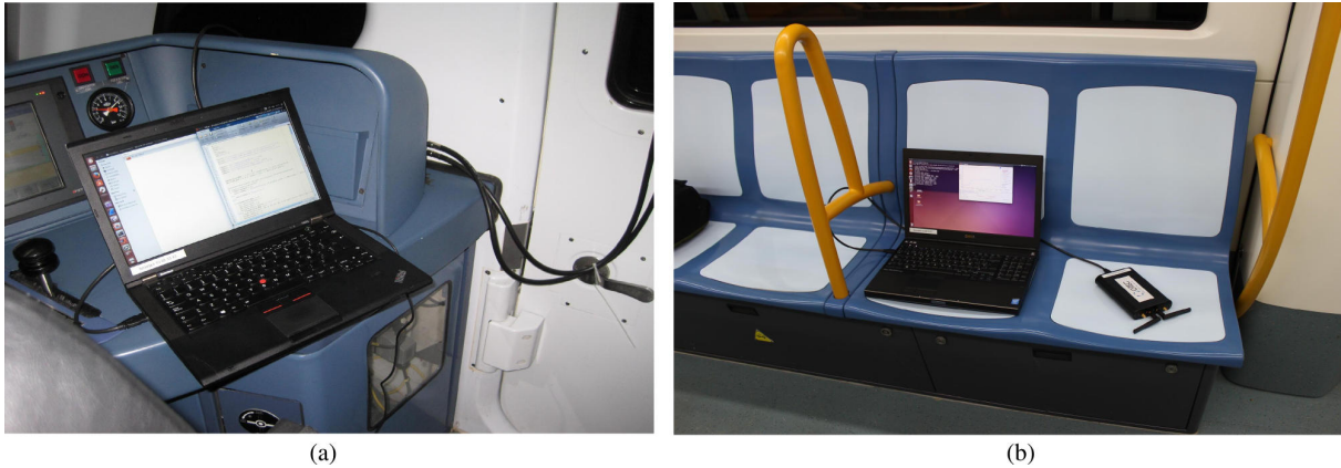
Figure 4.19: GTEC Testbed receiver nodes: (a) node connected to the outdoors antennas; (b) node provided with its own indoors antennas.
