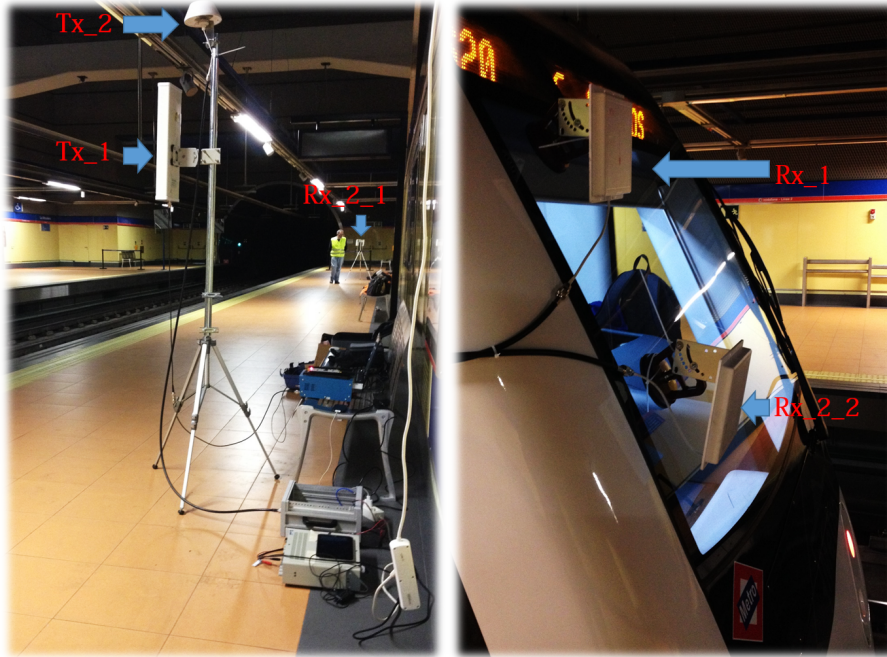
Figure 4.18: Deployment of the base station at the subway station as well as the outdoors receive antennas. The considered transmit antenna is labeled as “Tx_1”, while the outdoors receive antennas are “Rx_1” and “Rx_2_2”.
