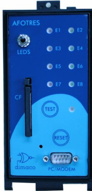
Figure 2.17: 8-loop vehicle inductive detector (Afotres-Dimaco).
