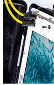
A rugged, portable unit with internal battery and waterproof connection plugs.
