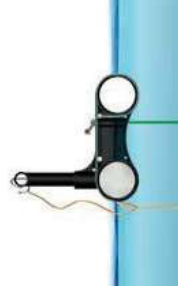
All the weight of the net and sinker tube system is supported by the floating pipe - NOT by the handrail.
