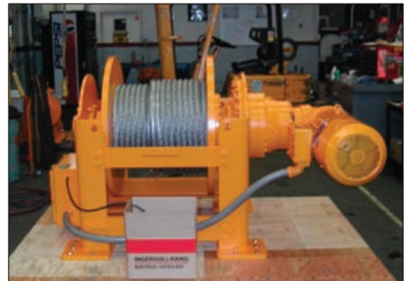
38,400 pound railway car moving winch
