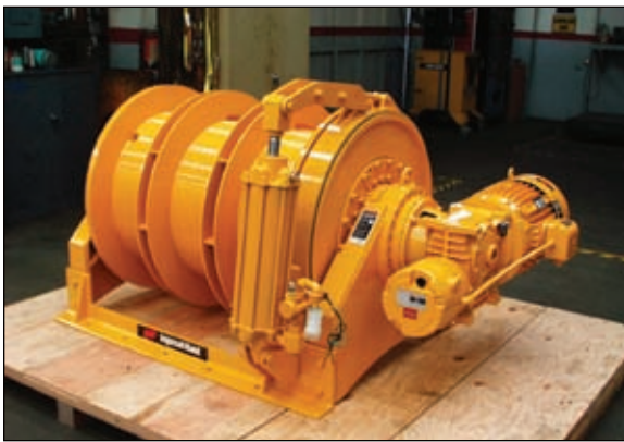
Custom launch vehicle payload handling winch
