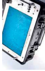
LCD screen made for rough, daily use and provides excellent readability in all light conditions.
