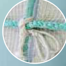
7. Double loops at the base where downward lines and cross ropes are connected. One loop is used for lifting the rope and the other for the weight system.
