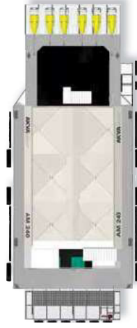
Machine room, silos aft deck
