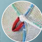
2. Red loops at the top of the waterline net connects the net to the cage. Red color means that this loop should NOT be used for lifting the net.
