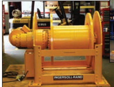
50,000 pound hose positioning winch
