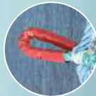
2. Red loops at the top of the waterline net connects the net to the cage. Red color means that this loop should NOT be used for lifting the net.
