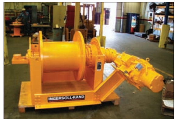
21,300 pound maintenance winch with dual brakes and vector duty motor
