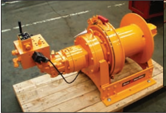
16,400 pound hydraulic pipe handling winch
