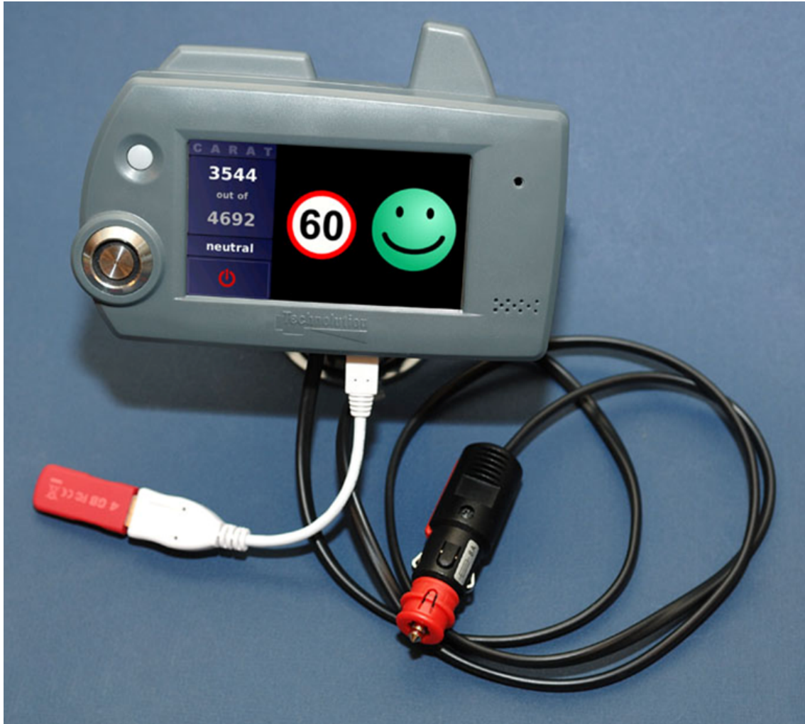
Figure 5.2: Field prototype of the CARAT counter, including the external shell with two buttons and a speaker, the display, the USB stick, the USB connector, and the cigarette lighter plug.
