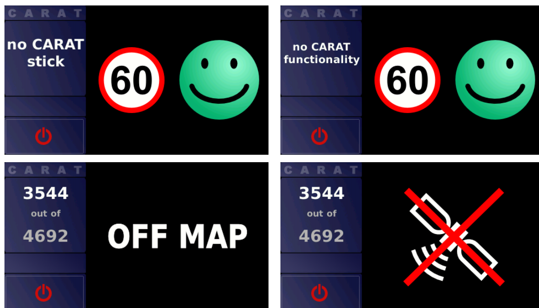
Figure 5.4: CARAT counter error alerts. Clockwise from top left: “no CARAT stick”, “no CARAT functionality”, “no GPS”, “off map”.
