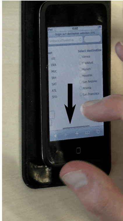
Figure 6.14: A small scroll bar appears at the bottom of the screen when the user presses and drags his finger
