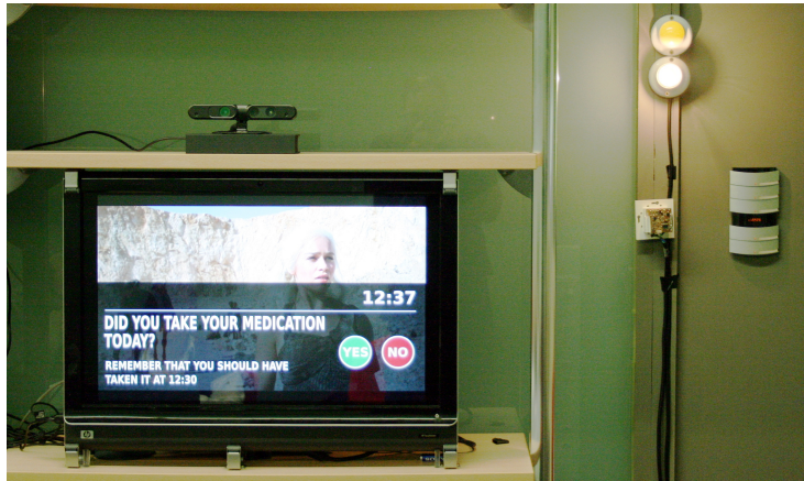
Figure 6.12: The OMNI UI adapted to the Deaf User scenario. The Kinect and the wall buttons can be used to control system (change channels, answer questions). The display is used to output notification messages, and the colored lights are used to request the focus of the user when a notification is displayed.
