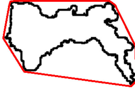
Figure 3.13: Convex hull area. Red line represents the smallest convex polygon that can contain the break-up contour.
