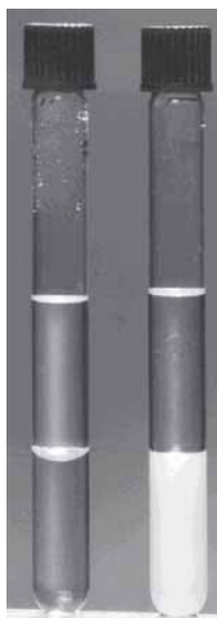
Figure 2. Hexadecane-water partition-test. Standard hydrophobic yellow 'sulphur flower' remains in the upper hexadecane-phase (left) whereas biologically produced sulphur remains in the lower water phase (right). (Taken from Janssen et al. , 1999).
