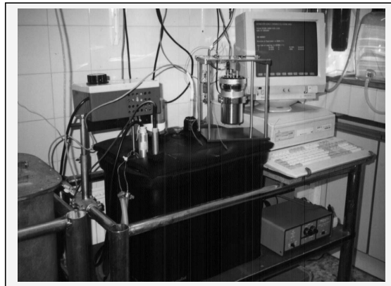
Figure 5. Bomb calorimeter assembly used by the Research Group TERBIPROMAT
