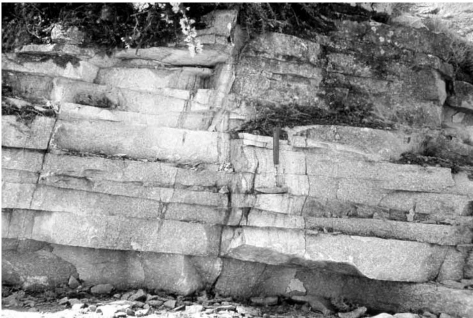
Fig. 3. Sheeting in granite rock intersecting the magmatic fabric (schlieren) from Mariz, Coruña Spain.
