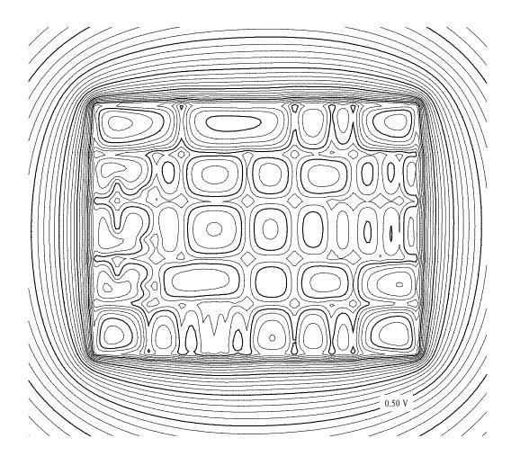
Figure 2.—E. Balaidos II Grid: Results obtained by BEM (1 parabolic element per bar). Ground surface potential distribution.
