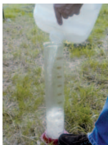
Figura 8. Probeta utilizada para realizar las mediciones de agua precipitada. Figure 8. Test tube used to perform measurements of precipitated water.
