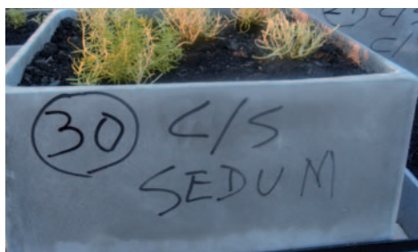
Figura 6. Detalle cubeta de 30cm de sustrato con Sedum . Figure 6. Tray detail with 30 cm of substrate with Sedum .
