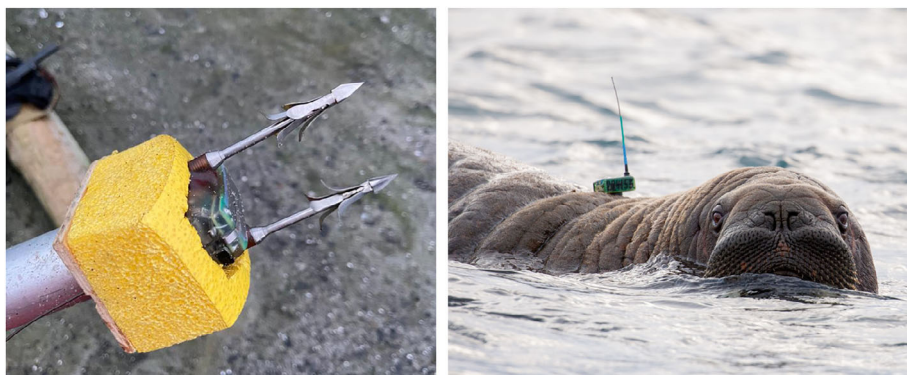
FIGURE 1 A platform terminal transmitter (SPLASH) on a harpoon (left); tagged walrus (Pulsar transmitter) in water (right).
