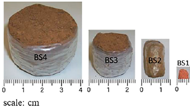
FIGURE 1 Four cylindrical undisturbed soil samples extracted from a soil block collected at 0–20 cm of a Brazilian oxisol (Rhodic Hapludox) with different diameters: 4 cm (BS4), 2 cm (BS3), 1 cm (BS2), and 0.5 cm (BS1).
