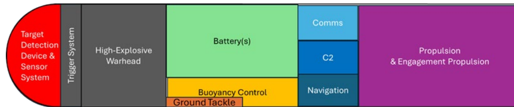
Figure 24. Physical Architecture of Sea Mine
