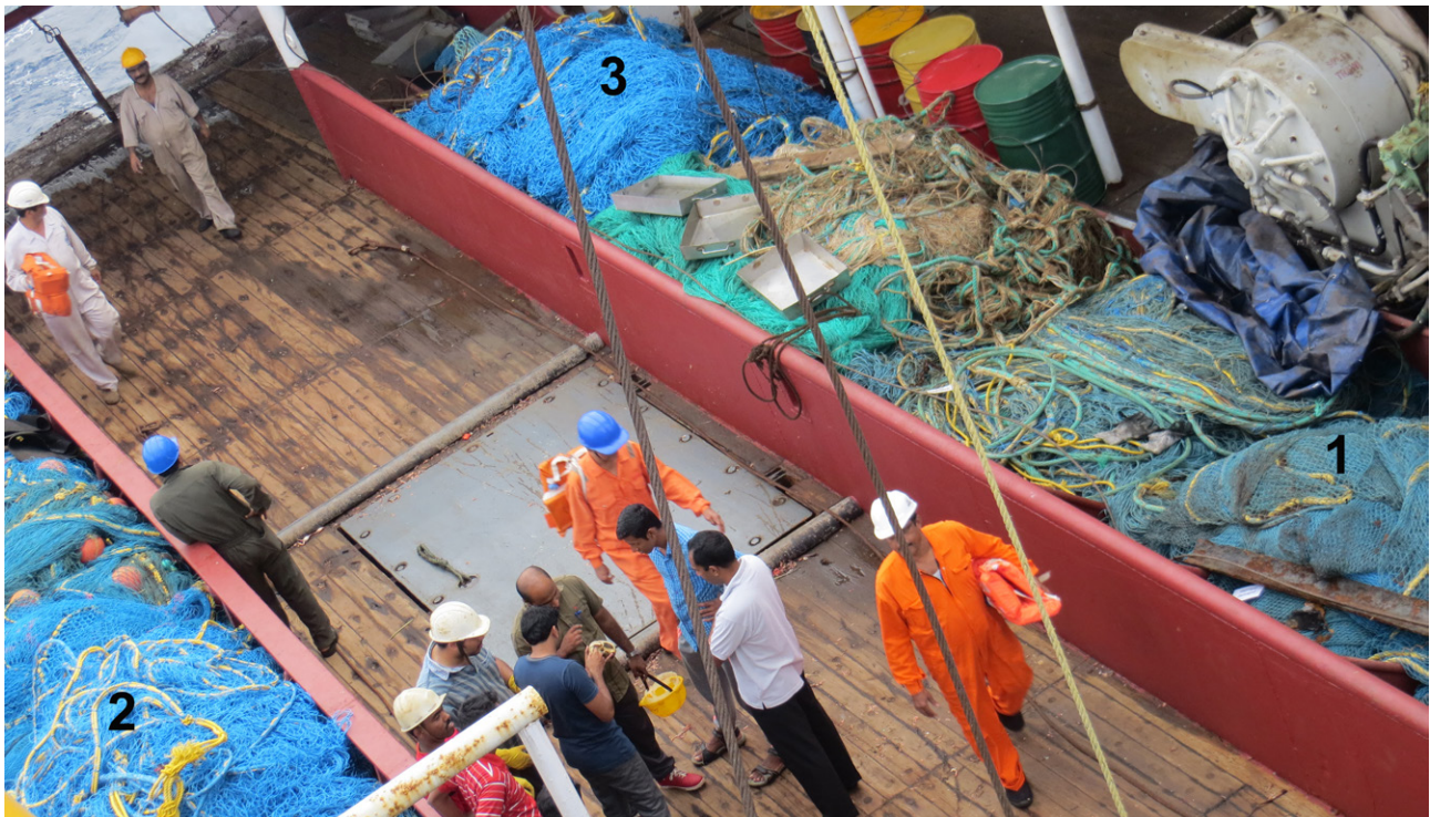
Three fishing nets evaluated during Deep sea fishing cruise 332- (1) EXPO model Fish trawl, (2) High Speed Demersal Trawl-Crustacean version HSDT- CV and (3) High Opening trawl (HOT) nets stored on the deck.
