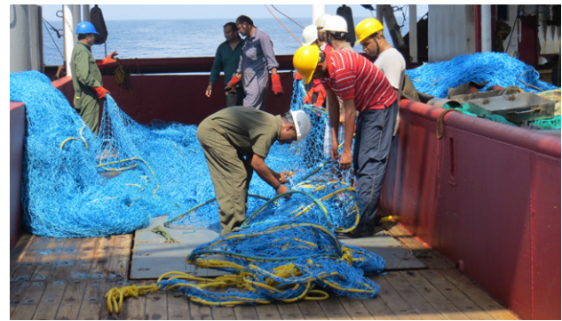
Rigging of the HOT trawl net with buoys in preparation for its first fishing trial in Cape comorin transect
