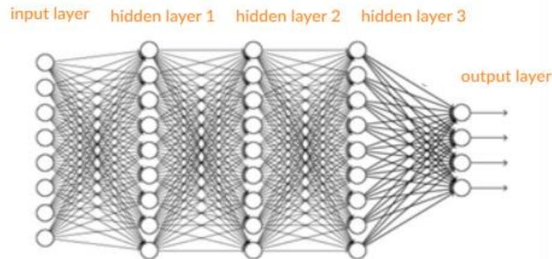
Figure 2. A deep neural network with three hidden layers.
