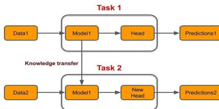
Figure 3. Architecture of Transfer Learning based models.
