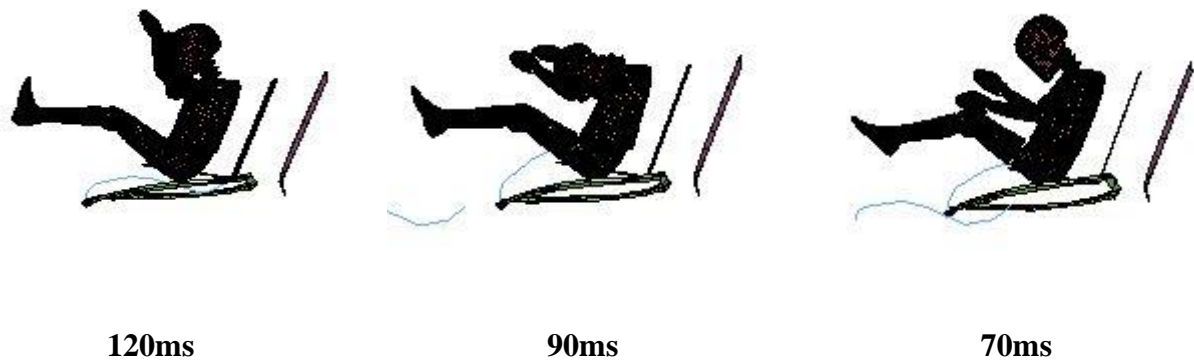
Fig. 3 The response of the dummy at instances in the crash simulation
