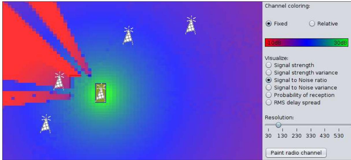
Figure 3(d). signal to noise ratio in colored radio channel around node surrounded with obstacle
