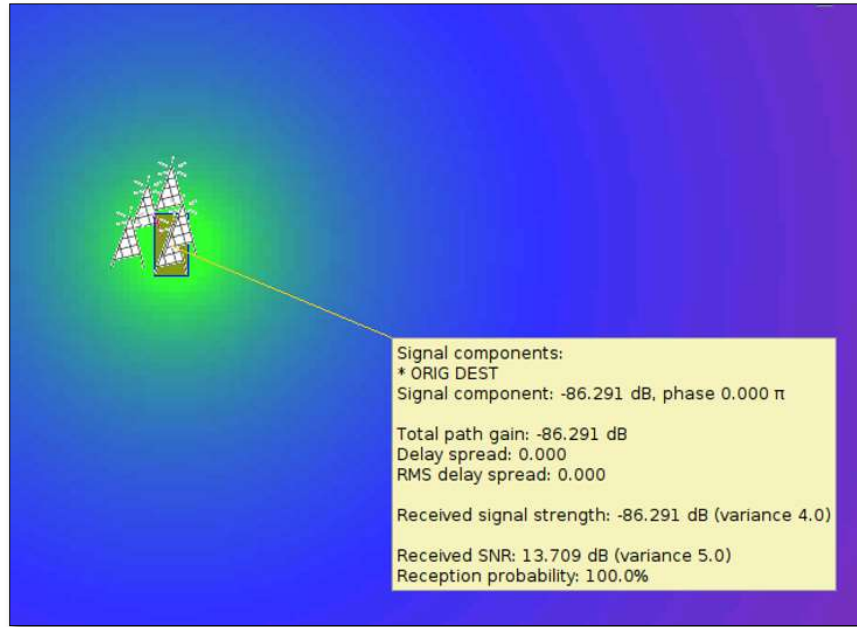
Figure 2(d). MRM signal reception at a distance of about 200 m away from the node
