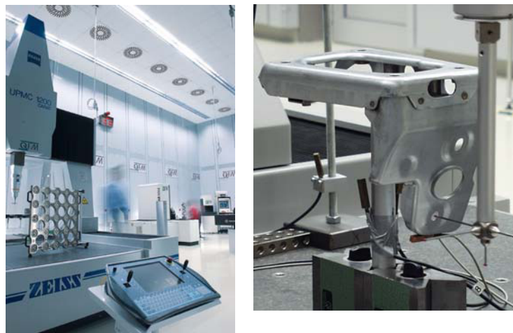
Figure 1. DKD calibration of a shaft collet with reference CMM
