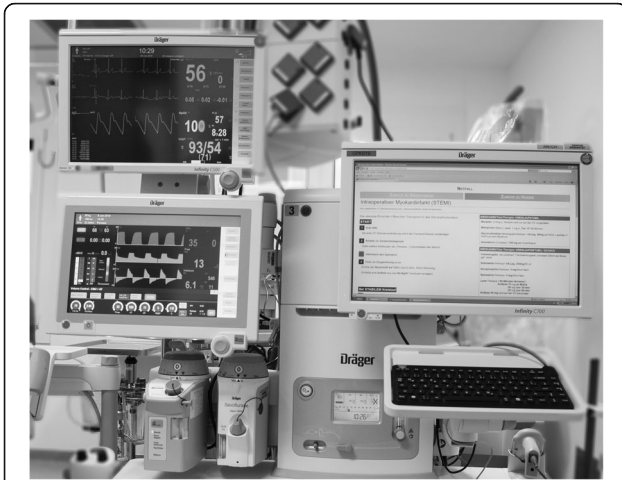
Fig. 2 Location of anaesthesia information management system with web-based cognitive aid. Placement provides easy accessibility and consistent location, without interfering with routine work flow . The layout was adapted from a paper based template available from Ariadne Labs [1]
