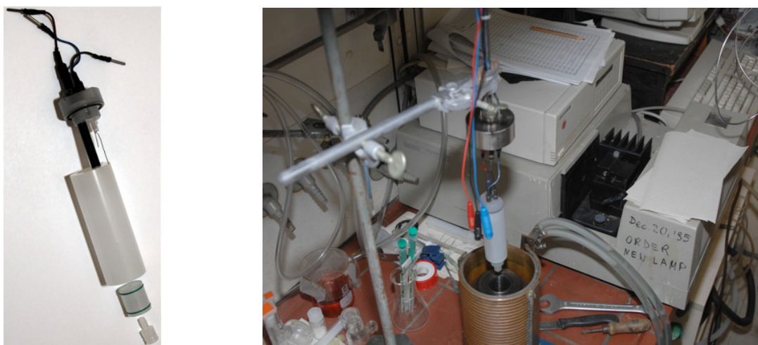
Figure 2.2. Left: the set of electrodes and Teflon cell body; right: the whole high-pressure electrochemical cell.
