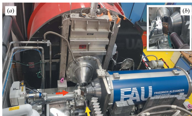
Figure 3 (a) Photograph of the SAXS instrument installed at the D22 instrument (ILL) for simultaneous SAXS/SANS experiment. (b) A sample at an angle of 45^\circ relative to both orthogonal neutron and X-ray beams. Lead shielding can be seen (1) on the front of the detector vacuum chamber, (2) along the neutron collimation and (3) on the side of the vacuum chamber of the X-ray detector. The red and yellow arrows indicate the directions of the X-ray and neutron beams, respectively.
