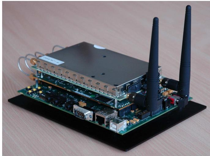
**Abbildung 4.9:** Lyrtech Small Form Factor Software Defined Radio Development Platform [68]
