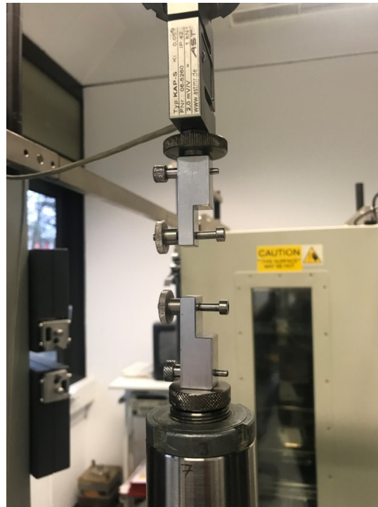
Figure 3. Experimental array for determination of the linear tensile strength of the suture materials.
