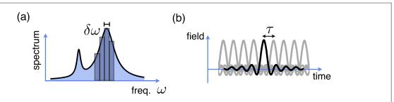
**Figure 2.** Wave packet picture that can be used in understanding the entanglement rate. (a) For each of the beams, we imagine to frequency-filter the field, with a filter size  $\delta\omega$ . (b) In time-space, this corresponds to wave packets spaced by  $\tau=2\pi/\delta\omega$ . These form a complete basis on a time–frequency grid. The use of a wave packet basis on a time–frequency grid in the context of quantum noise is reviewd in [35].
