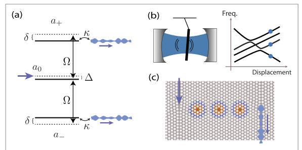
Figure 3. (a) Level diagram: the optical level distance almost matches the vibrational frequency  $\Omega$  so that phonon-mediated transitions between the optical levels occur. (b) Schematic for a possible implementation in a membrane-in-the-middle setup; three of the optical modes constitute an equidistant triplet for a suitable membrane position and tilt angle. (c) Schematic for the possible implementation in an optomechanical crystal, with one incoupling and one outcoupling waveguide.
