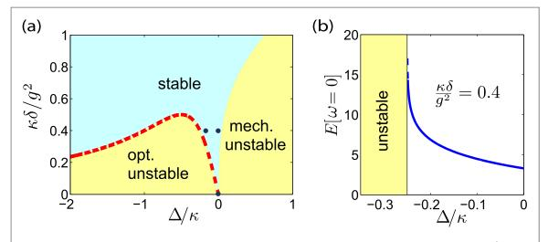
**Figure 4.** (a) Stability diagram of the model, versus frequency mismatch  $\delta$  and laser detuning  $\Delta$ , for  $g/\kappa = 5$  and  $\Gamma/\kappa = 10^{-3}$ . Stability boundary in the effective optical model: red dashed line. Parameter values corresponding to the (stable) blue points will be studied below. (b) Diverging entanglement from the effective optical model at the boundary of stability.
