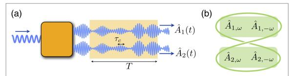
**Figure 1.** (a) A source of two entangled beams, where the aim is to calculate the entanglement between beams 1 and 2 in the large time interval *T*. (b) Frequency modes that are correlated (entangled) in the limit of large *T*.
