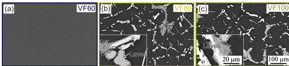
Fig. 5—Microstructures of the alloys (a) VF60, (b) VF80, and (c) VF100 after heat treatment at 1350 °C for 24 h and subsequent aging at 900 °C for 100 h at a low magnification show that additional phases in VF60 could be solved while \mu , \chi , and most likely Laves phases remain in VF80 and VF100.
