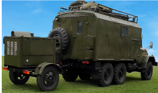
Fig. 1. MTO-AT mobile repair vehicle towing a power generator trailer
