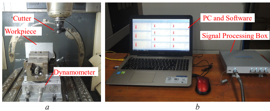
Fig. 6. Experimental system: a – cutting process components; b – signal collecting and processing
