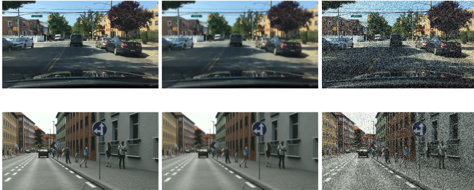
Fig. B.10.: Two exemplary object detection images from BDD100k (top row, real-world image) and SynScapes (bottom row, synthetic image), respectively. For each original image (left column), two corrupted versions are generated: a blurred one (middle column) and a noisy one (right column), see the text in Section 5.4 for details.
