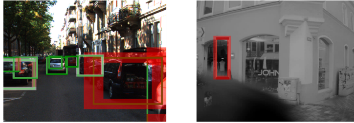
Fig. 1.3.: Visualization of (mostly) epistemic uncertainties in object detection. Each detected “traffic participant” corresponds to a rectangular frame. The thickness and color of the frame encode the respective position uncertainty, where green, thin frames indicate low uncertainty and red, thick frames imply high uncertainty. On the l.h.s., the detection of a dark car (the largest frame) is highly uncertain, likely because of the “novel” concept of an open trunk lid. On the r.h.s., the model confuses a mannequin with a pedestrian. Again, a high uncertainty estimate indicates the model’s lack of confidence. The left image is taken from the KITTI dataset (Geiger et al., 2012), with modifications from Pintz (2021), and the right one from the A2D2 dataset (Geyer et al., 2020), with modifications.
