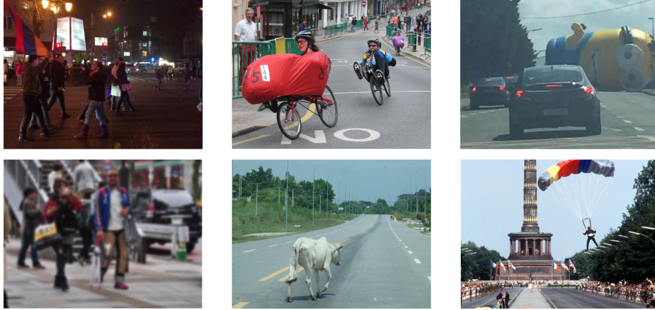
Fig. 1.1.: Examples of challenging and structurally new scenarios that an autonomous driving (AD) system may encounter during operations and that might cause insufficient or erroneous model behavior. The ability to detect such scenarios is crucial for safe AD, as it allows for activating redundant algorithmic systems or initiating a reduction of the vehicle speed. The displayed scenes differ in their probability of occurrence: while low contrasts and blurry sensor information (see left column) can be expected, not all types of traffic participants (see middle column) can be foreseen. Anticipating concepts that are unrelated to land transportation (like inflatable objects and parachutes, see right column) is almost impossible. The images are taken from various sources; see Challenging Traffic Scenes (2022).
