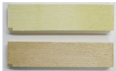
Figure 6. Pine wood and beech wood specimens coated with 1 wt. % of \text{TiO}_2 acrylic dispersion, [11].
