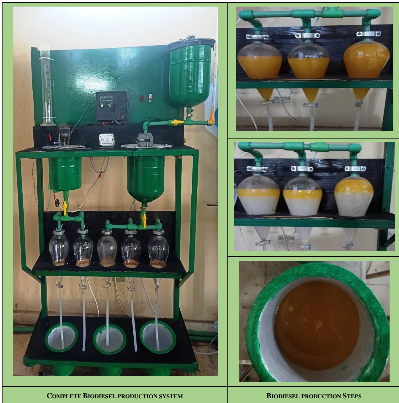
Figure 5. the actual image for the biodiesel test bench and produced WCO biodiesel.
