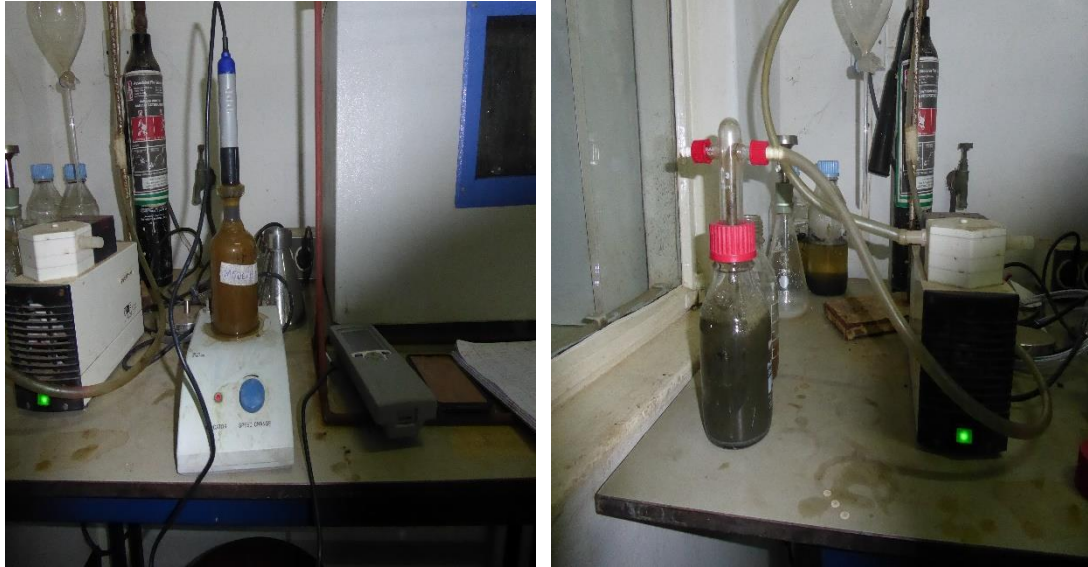
Figure 3-8: SOUR Setup (Left: SOUR Measurement using a DO meter probe; Right: Aeration of the sample before the performing the SOUR test) (Source: Author)
