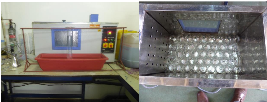
Figure 3-6: Water Bath used for the incubation of serum bottles at 35°C
