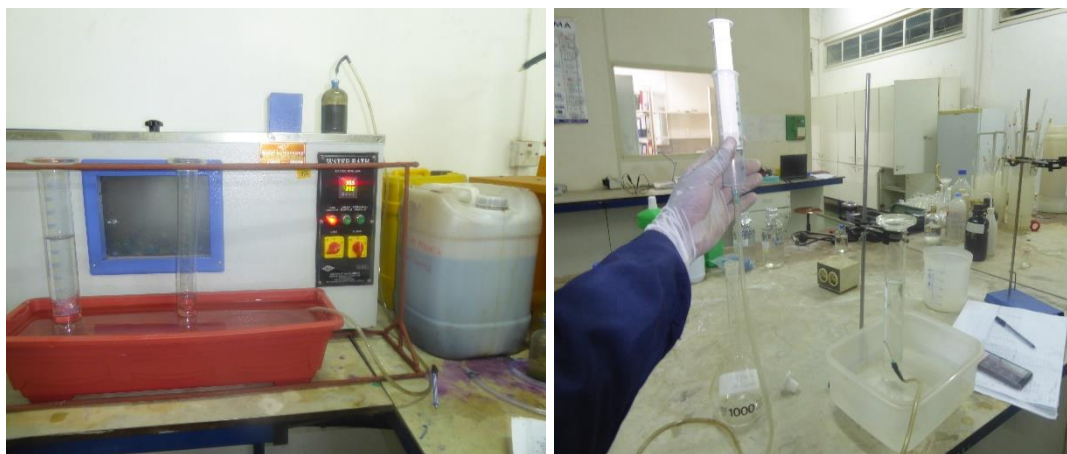
Figure 3-7: Gas Measurement using Liquid Displacement (LH: Biogas measurement; RH: Methane Content Measurement)(Source: Author)
