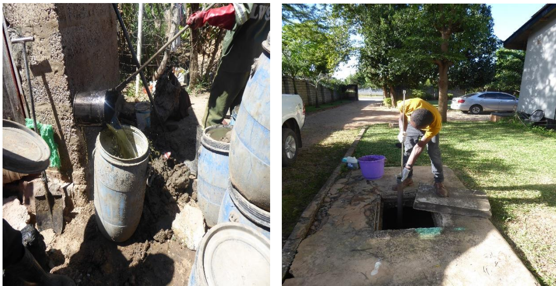
Figure 3-4: Faecal Sludge Sampling (LHS: Sampling from a pit latrine using an elongated scooper; RHS: Sampling from a septic tank using a core Sampler). (Source: Author)
