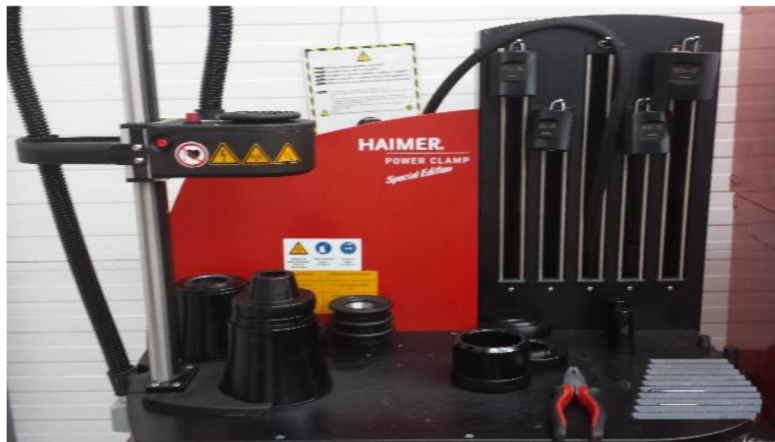
Figure 34 - Thermal heating machine for changes rotary burrs (DRT Moldes, 2012)
