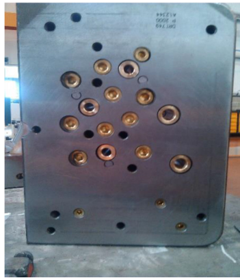
Bushing Channels sealed (DRT Moldes, 2012)
