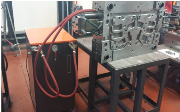
Water Leakage Test (DRT Moldes, 2012)
