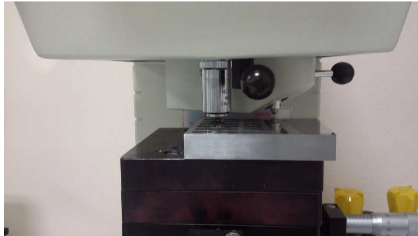
Figure 19 - Hardness Vickers Tester (SHIMADZU HMV/during the test process)
