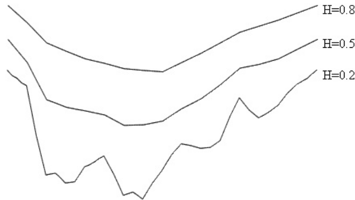
Figure 2.2: Execution examples of the random midpoint displacement algorithm
