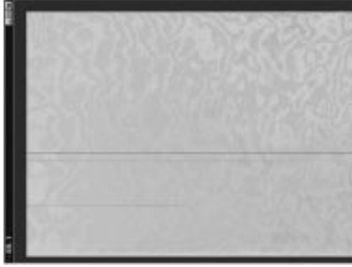
Fig. 3. Flat field of a OIG CCD obtained at 9000 Å. Interference fringes are clearly visible.
